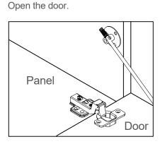
Adjust the door panelsupward or downward
