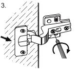
MOVE DOOR OUTWARD by turning this screw clockwise
