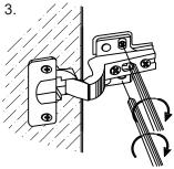
Unscrew 2 screws in round holes loosen 2 screws in oval holes a bit. Tighten 2 screws in oval holes. Screw in 2 screws in round holes
